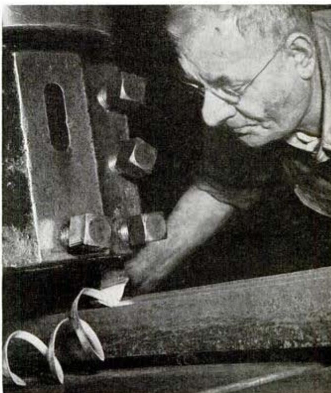
Molybdenum steel-tipped cutting tool shaving off layer of steel
